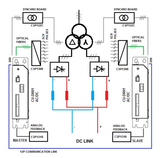
The two AC/DC converter bridges are composed by 6 thyristors each one connected in the B6C topology.
