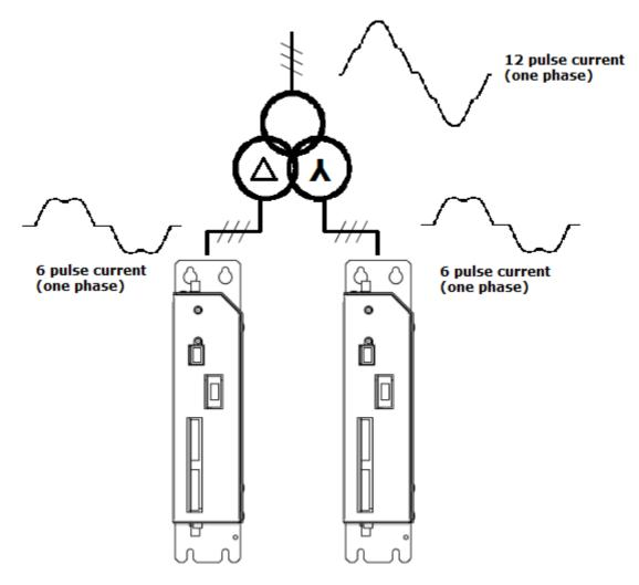
The most significant advantages of 12-pulse technology are:
